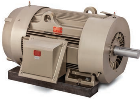
Conversion base allows any NEMA 449T frame to be mounted to an existing 586-8 frame
