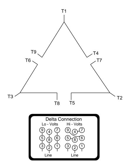
To reverse direction of rotation interchange connections L1 and L2.
