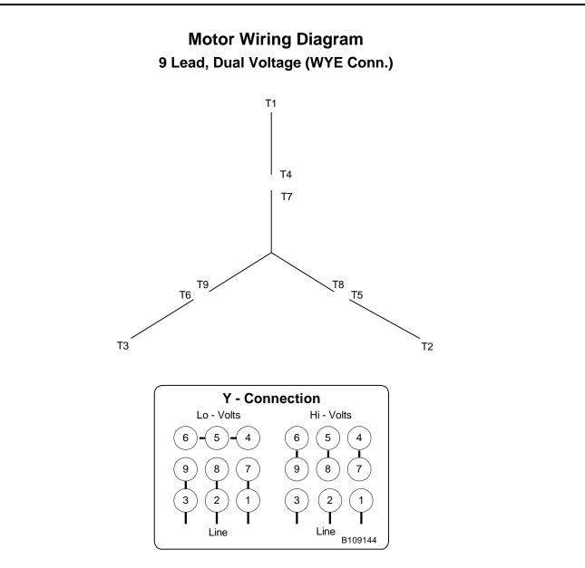
To reverse direction of rotation interchange connections L1 and L2.
