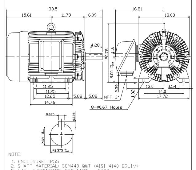
3. WITH THERMISTOR: PTC 140°C × 3PCS WIRED IN MAIN TERMINAL BOX
