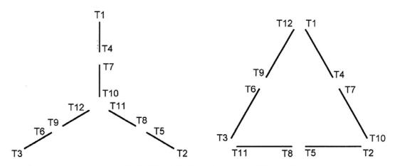
FULL VOLTAGE ACROSS THE LINE START AND RUN ON  $\Delta$  CONNECTION. ALSO SUITABLE FOR START ON Y RUN ON  $\Delta$ .
