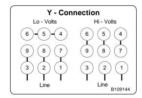
To reverse direction of rotation interchange connections L1 and L2.
