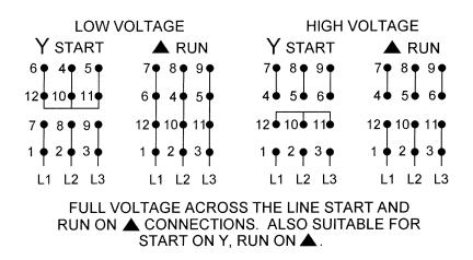
12 Lead, Dual Voltage, Wye Start / Delta Run, Both Voltages
