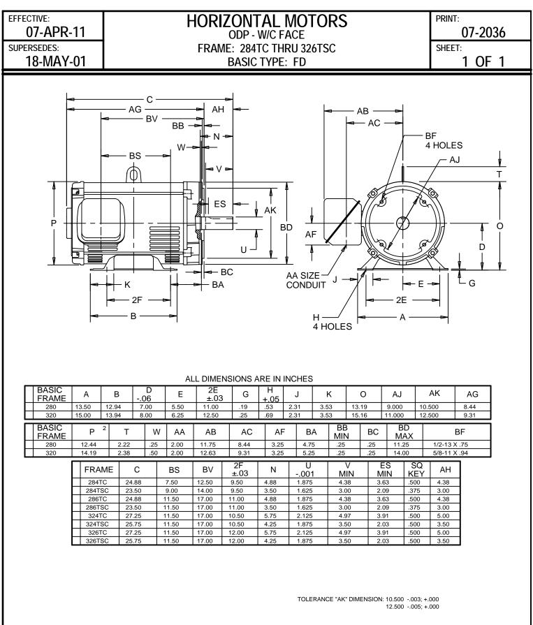
1: ALL ROUGH CASTING DIMENSIONS MAY VARY BY .25" DUE TO CASTING AND/OR FABRICATION VARIATIONS. 2: LARGEST MOTOR WIDTH. 3: CONDUIT BOX MAY BE LOCATED ON EITHER SIDE OF MOTOR. CONDUIT OPENINGS MAY BE LOCATED IN STEPS OF 90 DEGREES REGARDLESS OF LOCATION. STANDARD AS SHOWN WITH CONDUIT OPENING DOWN.
