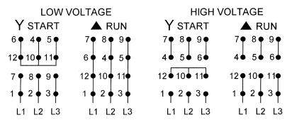
FULL VOLTAGE ACROSS THE LINE START AND RUN ON A CONNECTIONS. ALSO SUITABLE FOR START ON Y, RUN ON A.
