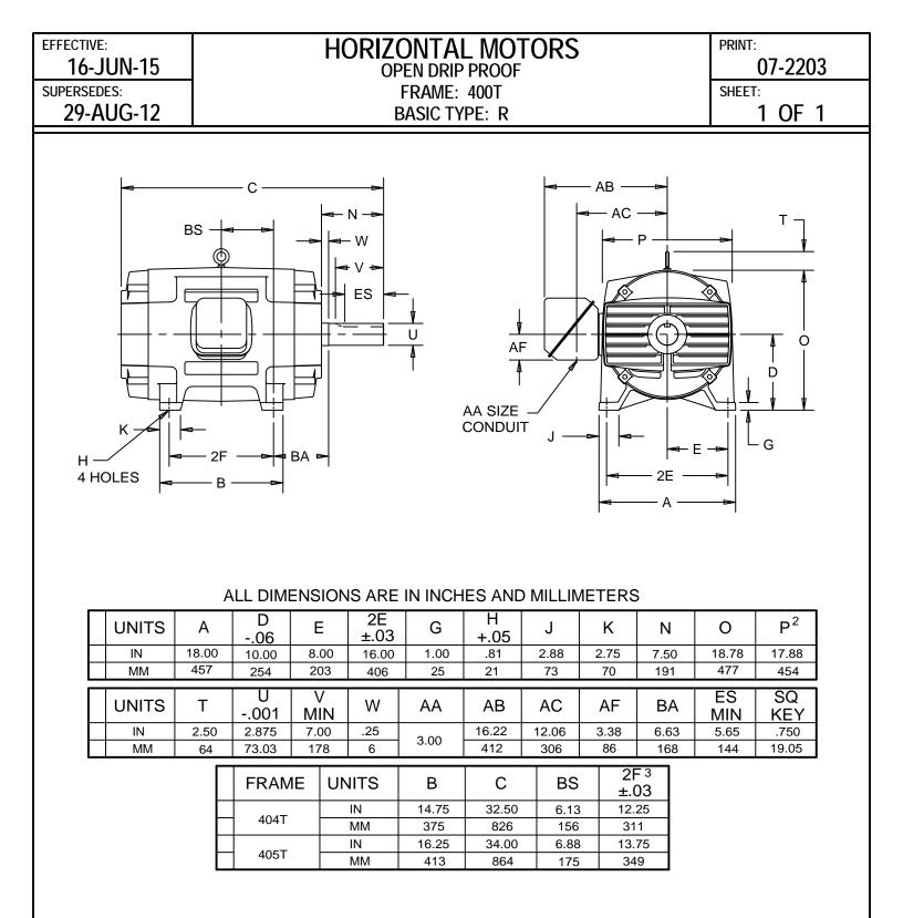
1: ALL ROUGH DIMENSIONS MAY VARY BY .25"(6mm) DUE TO CASTING AND/OR FABRICATION VARIATIONS. 2: LARGEST MOTOR WIDTH.
