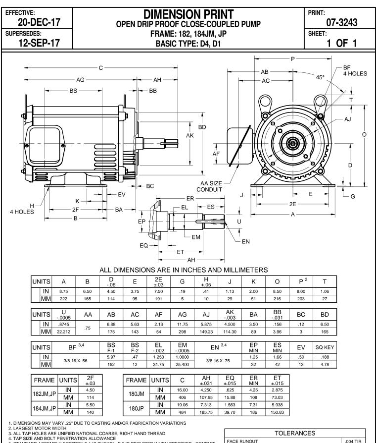
STANDARD ASSEMBLY POSITION F-1 IS SHOWN. F-2 IS PROVIDED WHEN SPECIFIED. CONDUIT OPENINGS MAY BE LOCATED IN STEPS OF 90° REGARDLESS OF THE LOCATION. STANDARD AS SHOWN WITH CONDUIT OPENING DOWN
