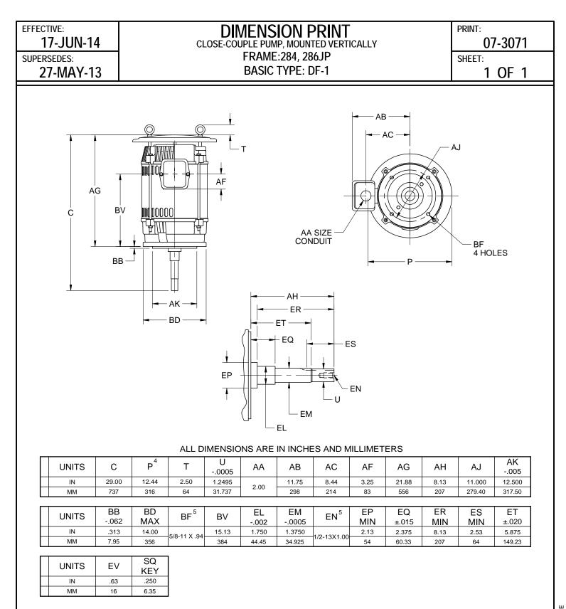
1. ALL ROUGH CASTING DIMENSIONS MAY VARY BY .25" DUE TO CASTING AND/OR FABRICATION VARIATIONS.
