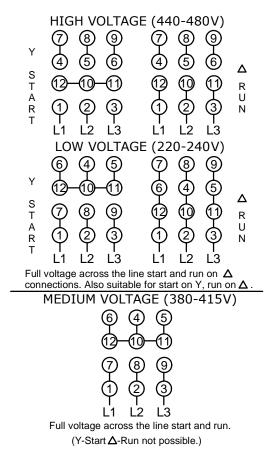
Per NEMA MG1 1998-1.76, "A Wye Start, Delta Run motor is one arranged for starting by connecting to the supply with the primary winding initially connected in wye, then reconnected in delta for running condition." This is accomplished by a special Wye-Delta starter configuration using twelve leads from the motor and is intended to limit the inrush current required to start the motor.
