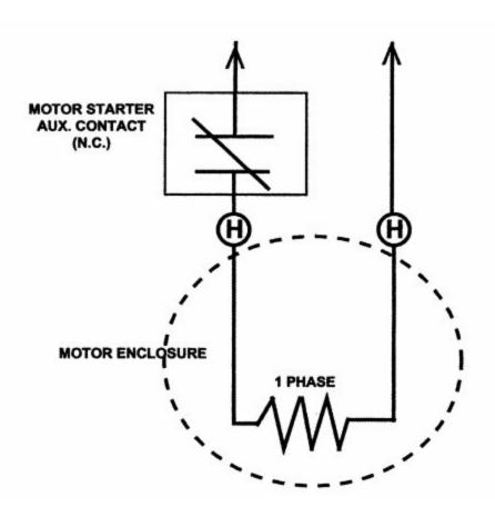
THIS EQUIPMENT IS SUPPLIED WITH ANTI-CONDENSATION HEATERS. HEATERS SHOULD BE ENERGIZED WHEN EQUIPMENT IS NOT OPERATING TO PROTECT UNIT BY PREVENTING INTERNAL CONDENSATION. CONNECT THE "H" OR HEATER LEADS TO
