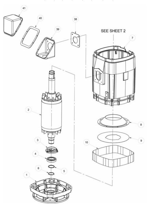
BEARINGS: Refer to motor nameplate for the bearing numbers.
