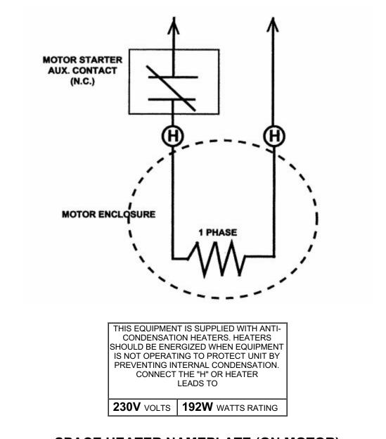
SPACE HEATER NAMEPLATE (ON MOTOR)
