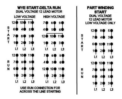
Per NEMA MG1 1998-1.76, "A Wye Start, Delta Run motor is one arranged for starting by connecting to the supply with the primary winding initially connected in wye, then reconnected in delta for running condition." This is accomplished by a special Wye-Delta starter configuration using six leads from the motor and is intended to limit the inrush current required to start the motor.
