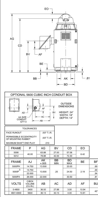
1. DIMENSIONS MAY VARY .25" DUE TO CASTING AND/OR FABRICATION VARIATIONS. 2. DIMENSIONS AND TOLERANCES ARE SHOWN IN INCHES.
