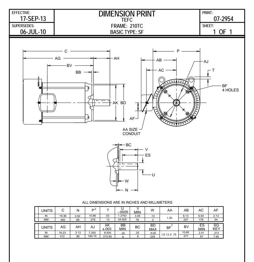
1: ALL ROUGH DIMENSIONS MAY VARY BY .25" DUE TO CASTING AND/OR FABRICATION VARIATIONS. 2: LARGEST MOTOR WIDTH.
