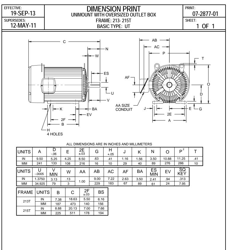
1: ALL ROUGH CASTING DIMENSIONS MAY VARY BY .25" DUE TO CASTING AND/OR FABRICATION VARIATIONS.
