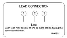
To reverse direction of rotation interchange connections L1 and L2.
