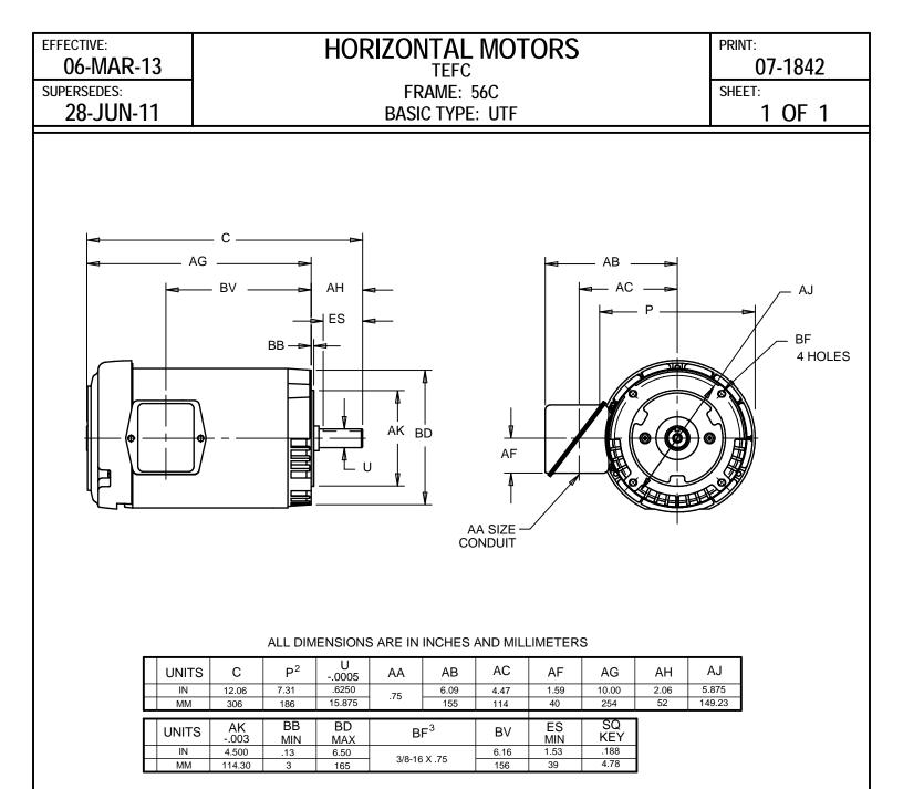
1: ALL ROUGH DIMENSIONS MAY VARY BY .25" DUE TO CASTING AND/OR FABRICATION VARIATIONS. 2: LARGEST MOTOR WIDTH. 3: TAP SIZE AND BOLT PENETRATION ALLOWANCE.
