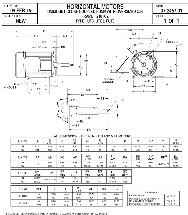
ALL ROUGH DIMENSIONS MAY VARY BY .25" DUE TO CASTING AND/OR FABRIO 2. LARGEST MOTOR WIDTH.
