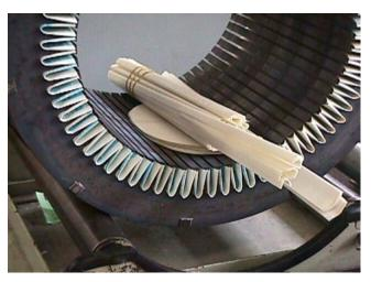
Premium Electricial Steel for improved efficiency, reliability and repairability, C4 coated silicon steel can withstand burnout oven temperature of 500°C (932F) minimum, to insure motors can be rebuilt to original performance.
