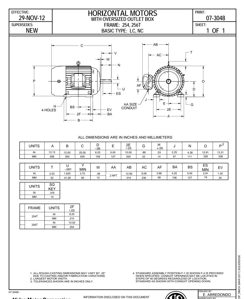
1. ALL ROUGH CASTING DIMENSIONS MAY VARY BY .25" DUE TO CASTING AND/OR FABRICATION VARIATIONS. 2. LARGEST MOTOR WIDTH.
